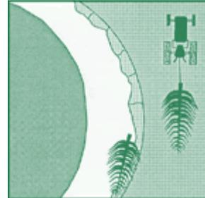
**3.** Tree is pulled tightly against bank and anchored at points shown by arrows
